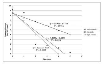
Figure 1. Regression lines equations describing the dynamics of *Salmonella* population during mesophilic anaerobic digestion
